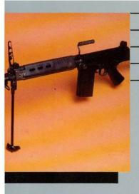
FAL Automatic Rifle is a gas operated weapon which shows closed bolt and it is positively bolted. It is a light weapon and it allows the immediate performance of an intense fire. It is usually operated on semi-automatic mode (single shot). The automatic shot can be performed under good conditions of stability.
